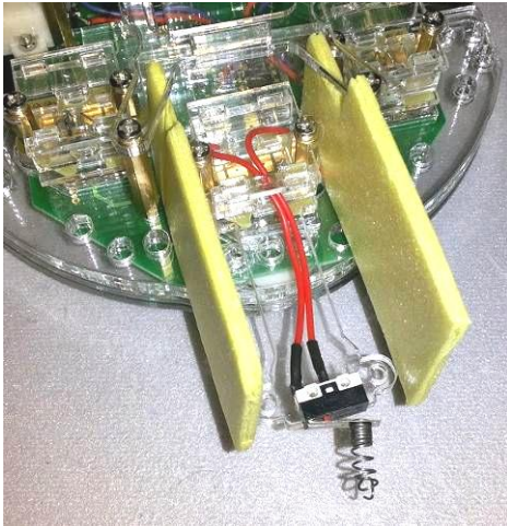
Fig. 56. The line probe with a bumper, and the blinders for the light sensors.
