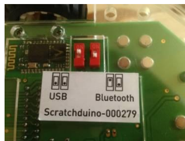
Fig. 15. Position of the jumpers for Bluetooth connection.
