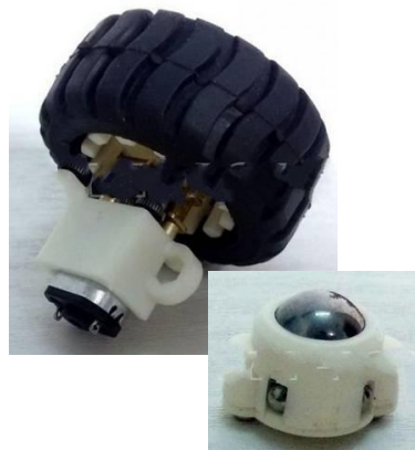
Fig. 44. Motion devices: a reduction motor with wheel and a ball bearing.
