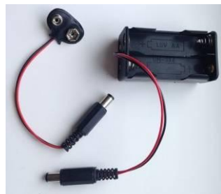
Fig. 13. A clamp for 6F22 battery and the housing for four AA batteries.
